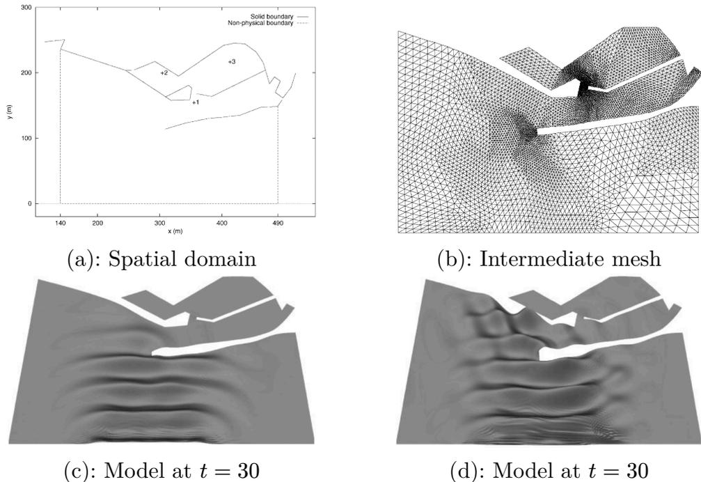
Figure 1: Unstructured triangular meshes of the harbor geometry (a, b) and simulated model of the the waves on the free surface at time  $t$  (c, d) [1].
