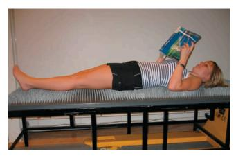
Recall that pressure is defined as p = F/A, so rearranging, we can calculate the maximum safe force of a single nail can support
