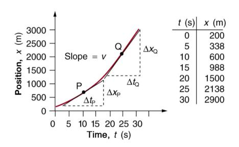
Example. Find the velocity of jet at t = 25 s by finding slope.
