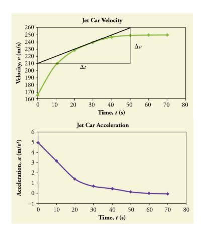
Example. Find the accel. of jet at t = 25 s by finding slope.
