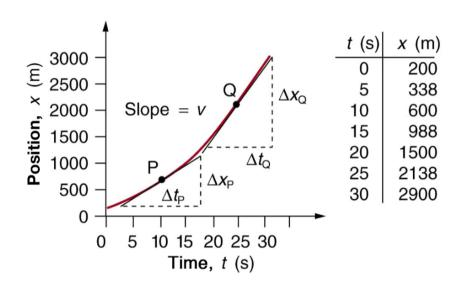
Example. Find the velocity of jet at t = 25 s by finding slope.
